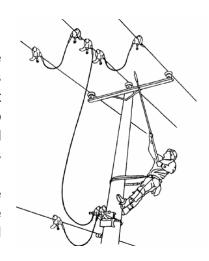
For electrical workers, we install grounds for two reasons. By installing grounding jumpers in a grounded and short-circuited configuration we ensure that the circuit is de-energized (removed from the source) and if the circuit was to accidentally become re-energized, the current sensitive devices we mentioned earlier will be activated. The design intent of those devices is to remove the circuit or equipment from the source of potential by providing an open point.
