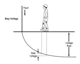
Be aware of the hazards of Step and Touch Potential. No matter what temporary grounding method is used, workers on the ground could be exposed to hazardous potential differences.
