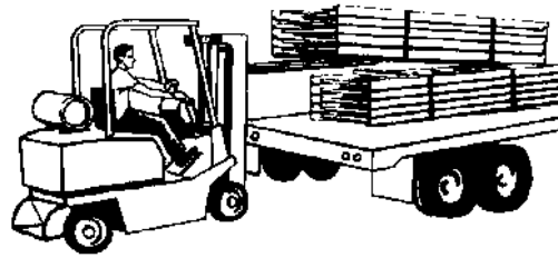
Figure 1-2—Incorrect (Except when Using Extended Forks for Skidded Bundles)
