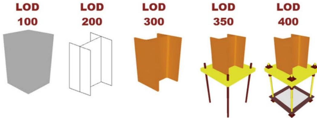
By using LOD, teams across multiple trades can communicate with each other with clarity and eliminate discrepancies in getting a project completed. Handling and interpreting a BIM model can be challenging, especially since it is easy to interpret the definition of details and completion on a project differently. LOD enhances clarity and serves to help improve understanding and communication on the scope of the final BIM deliverable.
