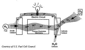
The anode side of the fuel cell receives the hydrogen and oxygen (from air) enters the fuel cell through the cathode. The catalyst splits the hydrogen atom into a proton and an electron, with each taking a different path to the cathode. The electrons create a separate current that can be utilized and the proton passes through the electrolyte. At the cathode both are reunited with the hydrogen and oxygen in a molecule of water.
